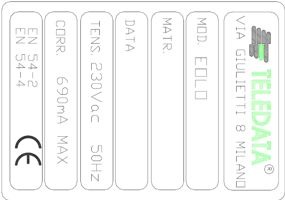
label of control panel
