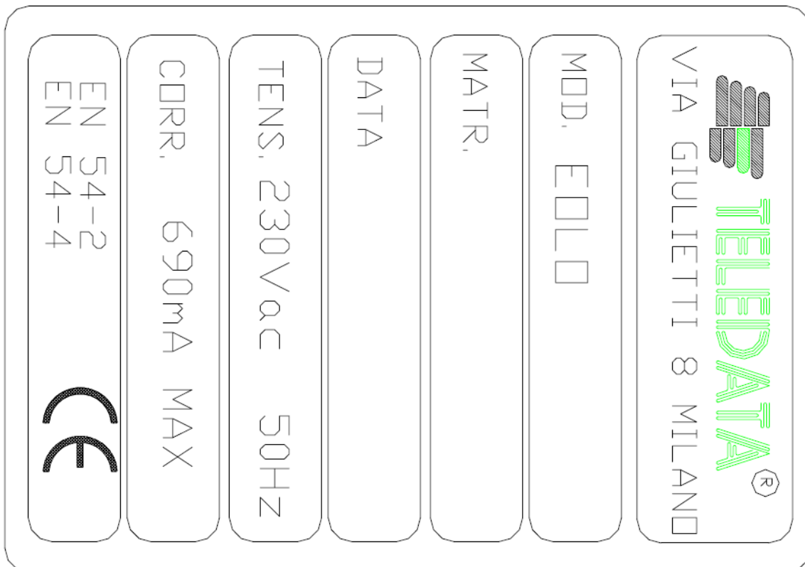
label of control panel
